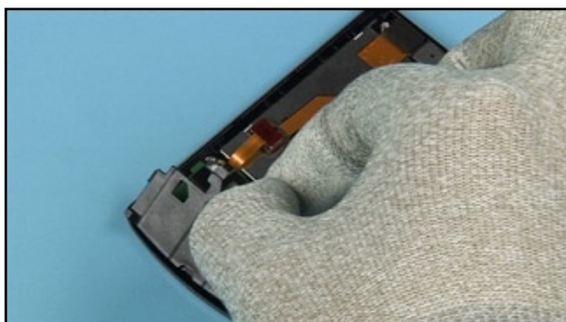
30. Insert the TOP KEYMAT SUPPORT, beginning from the top.
